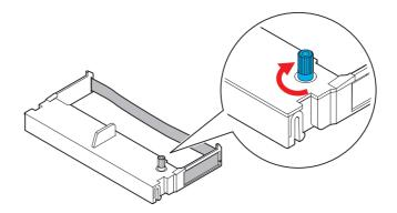
**5** Insert a new ribbon cartridge until it clicks into place. If there is slack or a fold in the ribbon, reinstall it.
