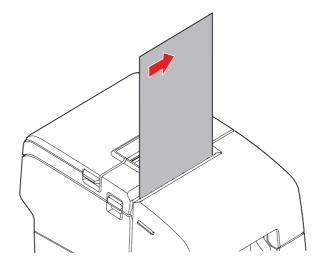
3 Insert the paper straight down until the bottom edge of the paper touches the stopper.
