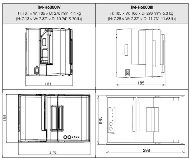
The figures above are those of the standard model with the MICR reader and E/P. Excluding the connector cover.
