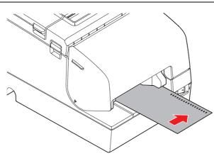
3 Insert the paper straight until the top edge of the paper touches the stopper.
