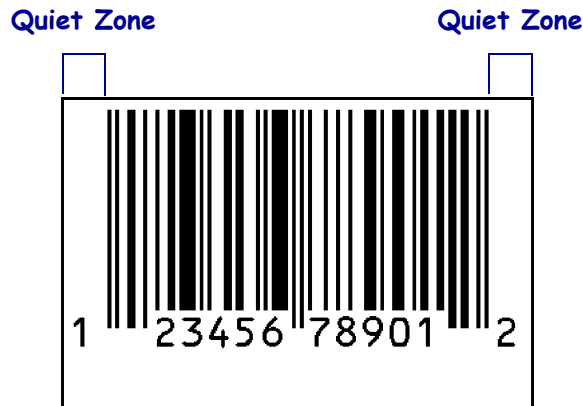
Figure 9 • Quiet Zone in a Bar Code
